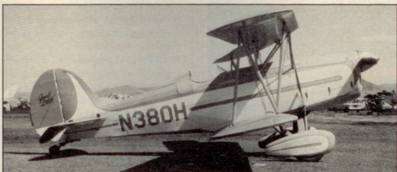
Clyde Parsons owned serial number 15. It had one engine swap—to a 150-hp Menasco. He increased the original small tail and changed the engine to a 200-hp Ranger.
