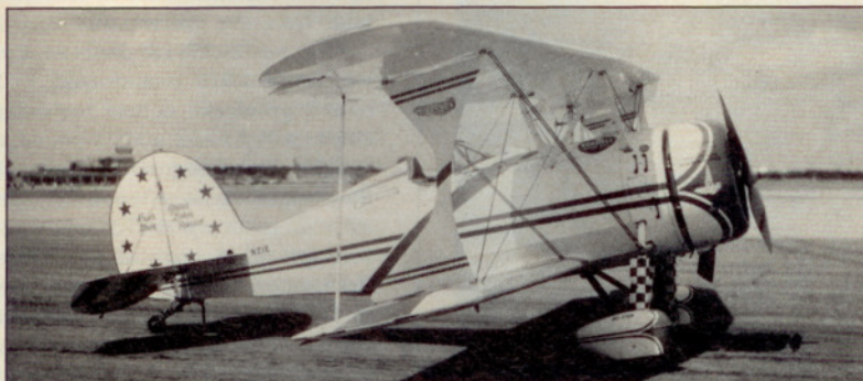
Harold Krier's highly modified Great Lakes was a regular at air shows and competitions for years. He added 1 struts, ailerons to the upper wings and more landing wires.
